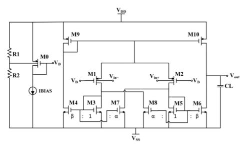
Figure 3. Schematic of the OTA with positive feedback proposed in [29].
