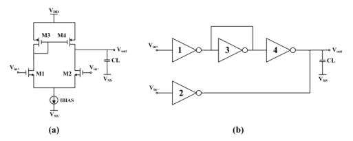
Figure 6. Conventional (a) and inverter-based (b) single-stage OTA.
