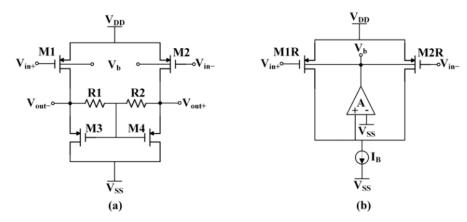
Figure 4. (a) Minimum-supply differential pair (b) common-mode control circuit proposed in [31].
