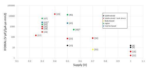
**Figure 16.** *IFOM* $_{AL}$  vs. supply voltage (\* simulated).
