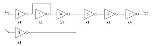
Figure 7. Schematic of the inverter-based OTA in [43].
