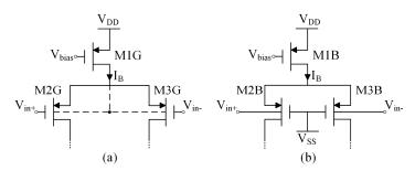
Figure 2. (a) Gate-driven and (b) bulk-driven p-channel differential pairs.
