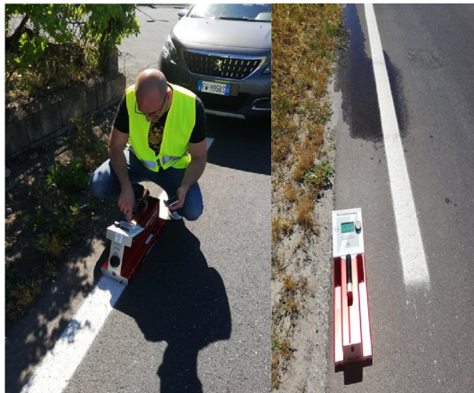
Fig. 3 – Survey of the marking retroreflectance in dry (RL, Qd) and wet conditions (RLw).
