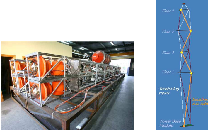
Fig. 6. Left: The mini-tower completely integrated at the Port of Catania. Right: A scheme of the mini-tower unfurled.
