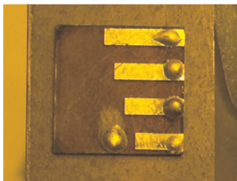
FIGURE 8 A device containing four organic solar cells [Color figure can be viewed at wileyonlinelibrary.com ]
