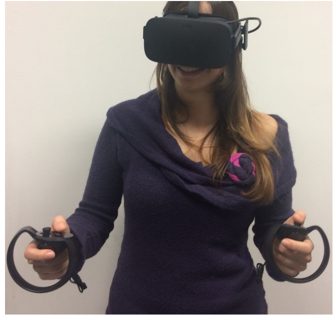
Fig. 4. Player using the Oculus Rift (VR headset) and the input peripherals.
