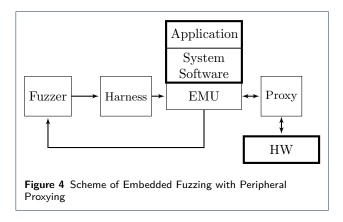
When deep knowledge about the SUT is missing, hardware accesses of the firmware must be treated differently. An alternative solution is to forward each hardware access to the real device. Therefore, a proxy application is introduced to route appropriate values and triggered interrupts between the actual hardware and the emulation, as shown in figure 4.
