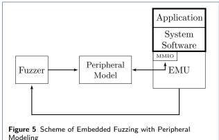
When implementing virtual hardware takes too much effort and peripheral proxying is too slow for fuzzing, the automated hardware modeling can be a solution. The idea is to learn how to respond to hardware accesses such that the firmware continues its execution. The peripheral model is thereby directly connected to the MMIO address space and can be supported by the fuzzer, as depicted in figure 5.
