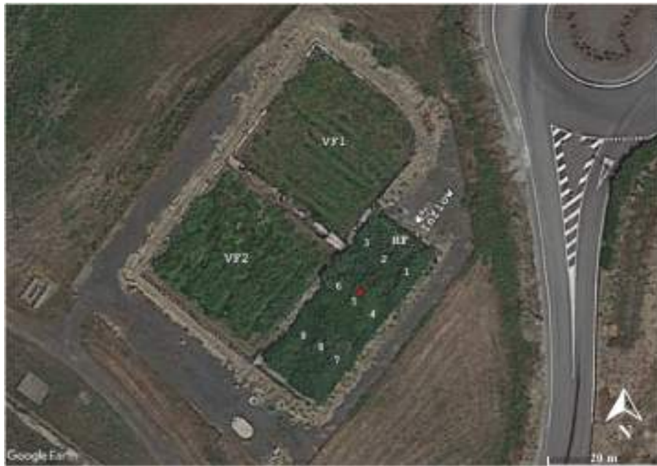
Fig. 8. IKEA Store hybrid treatment wetlands (Catania, Sicily; 37° 26' 48.30" N, 15° 1' 56.44" E, WGS84). The red cross is the CO 2 sampling point in the HF unit (numbers are the piezometers that divide the unit in three transects: points 1–2–3 indicate the first transect; points 4–5–6 the second transect; points 7–8–9 the third transect). VF1, VF2 are the two vertical subsurface flow wetlands.
