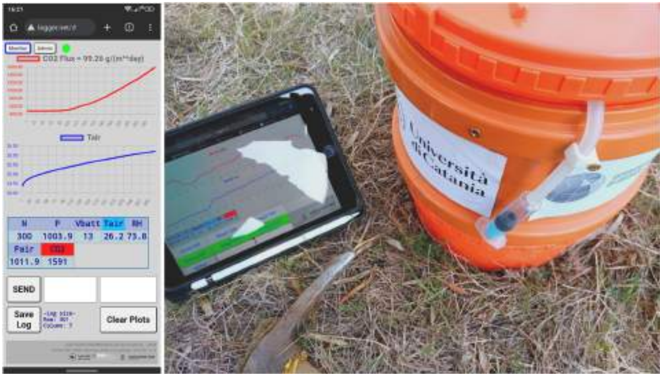
Fig. 2. Web application user interface; smartphone screenshot (a) and on a tablet during in-field operation. The upper green circle is a flashing heartbeat indicator for WebSocket connection status.
