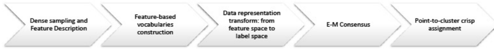
Figure 2.5: The pipeline implemented to represent images using Consensus Vocabularies and crisp point-to-cluster assignment.
