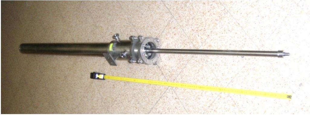
Fig 2. The adopted mechanical extendible handler
