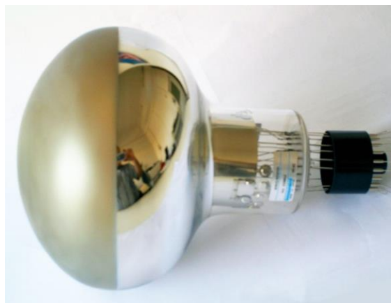
Fig 9. The PMT Hamamatsu R5912-MOD.
