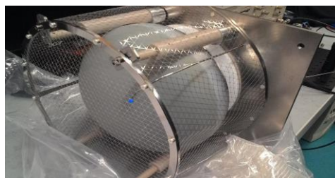
Fig 21. Picture showing the stainless steel pipe which drives the end section of the calibration optical fiber toward the PMT window. A blue-light laser spot on the PMT surface can be noticed.
