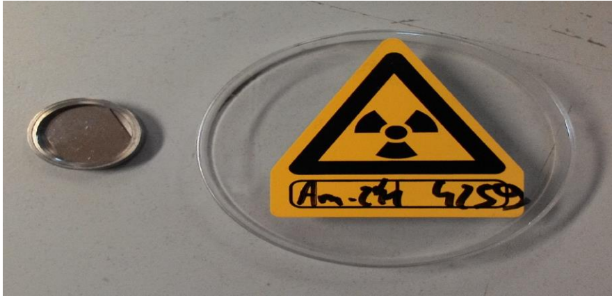
Fig 3. Picture of the used alpha source
