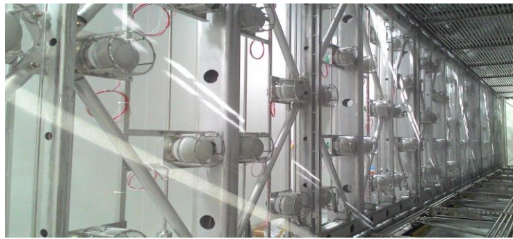
Fig 8. Scheme of the adopted geometry with 90 PMT's behind each wire plane and picture of the actual configuration.
