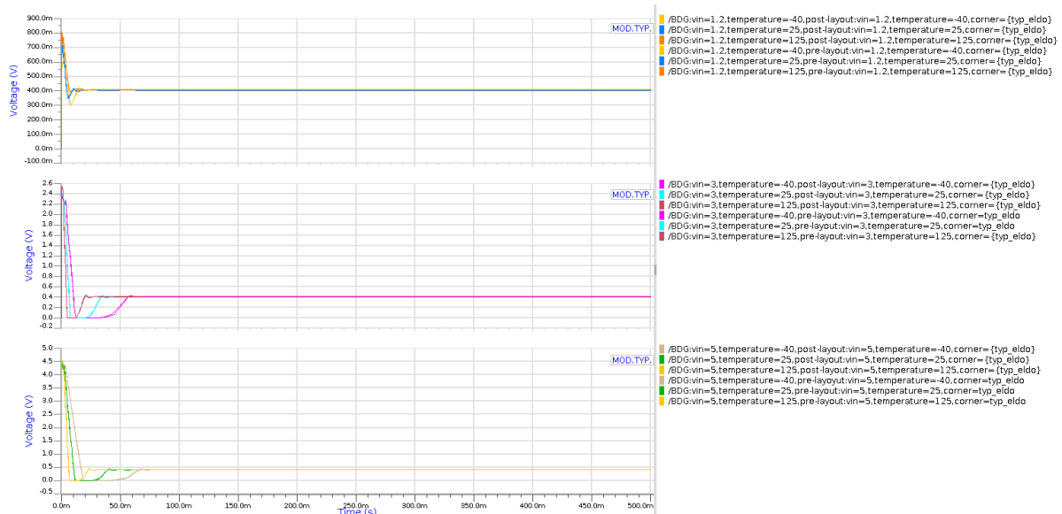
Fig. 73. Post-layout simulation results of the transient response of the V_{BDG} at the start-up for different value of supply voltage and temperature (MOD. TYP.).
