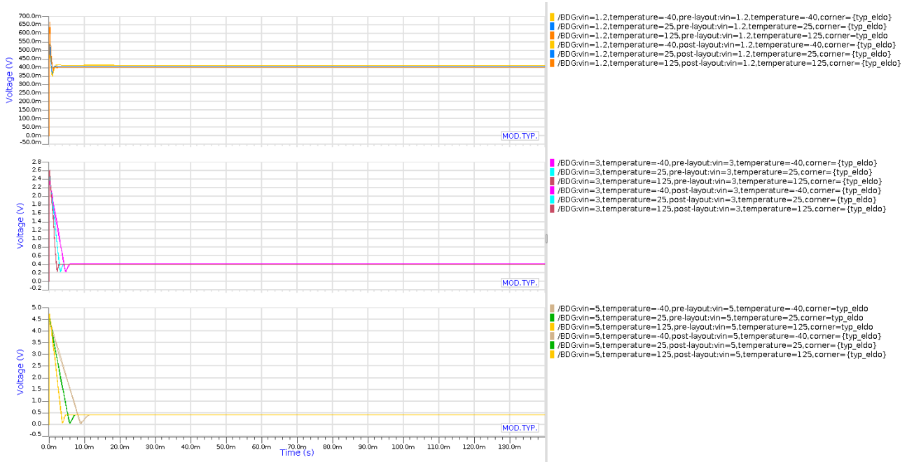
Fig. 93. Post-layout simulation results of the transient response of the V_{BDG} (8 nA version) at the start-up for different value of supply voltage and temperature (MOD. TYP.).
