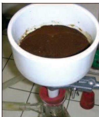
Figure 29-Filtration under vacuum of LV pellets
