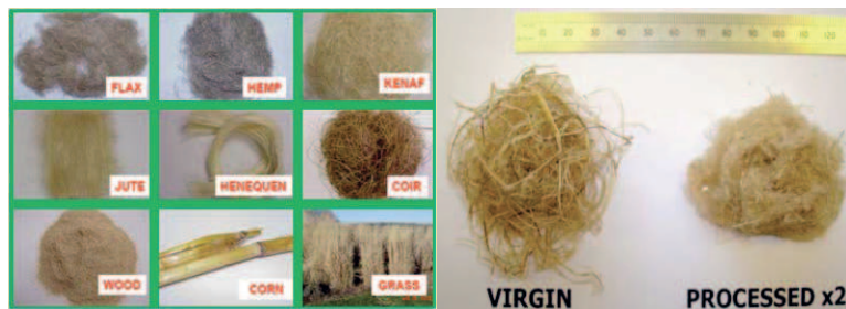
Fig. 4. (a) Some natural fibre, (b) Processed hemp fibre (source: University of Exeter)
