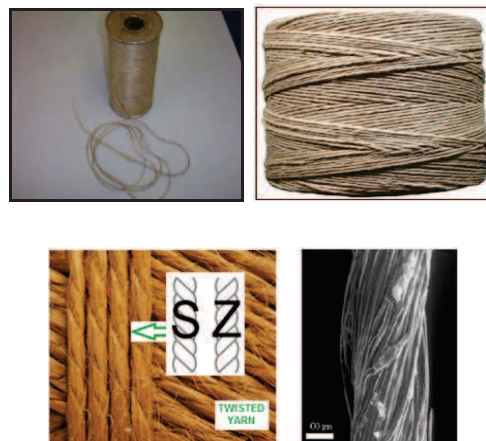
Fig. 9. Hemp twisted yarn and scanning electron microscope image of hemp twisted yarn.
