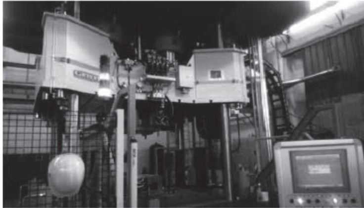
Figure 33- Cannon Afros plant used for HP-RTM trials (1000tons press and high pressure metering mixing unit).
