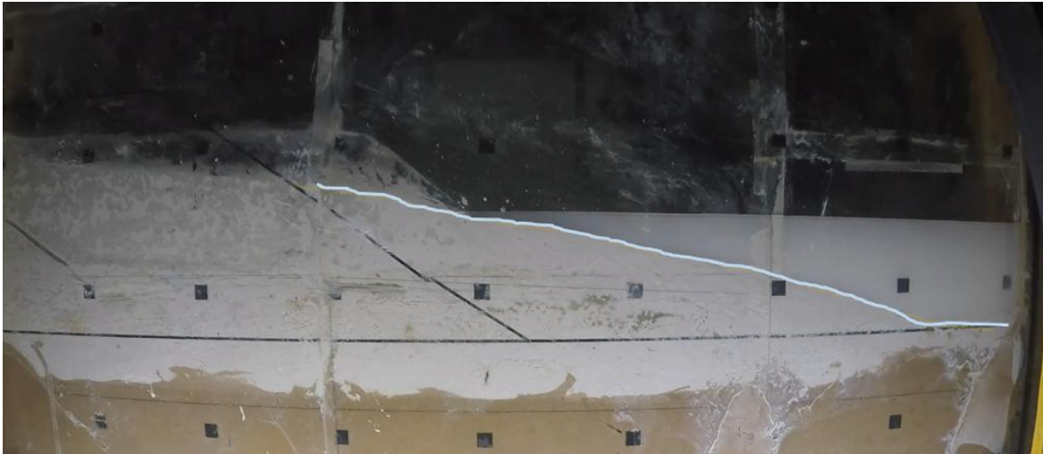
Figure 33. Time-lapse slope deformation through contour overlays from t_9 (50g) until the end of the test t_{11} . Continuing with the rain simulation.
