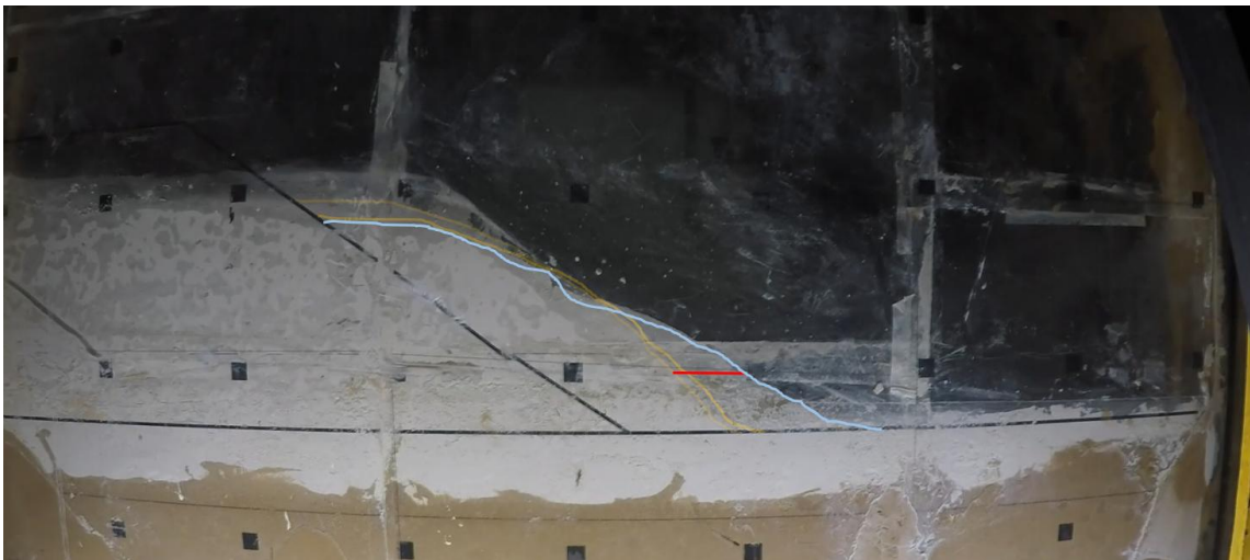
Figure 28. Time-lapse slope deformation through contour overlays from t_4 (15g) until before reaching the t_5 (20g).
