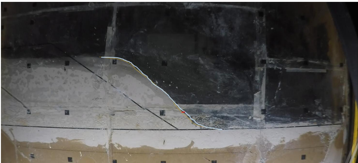
Figure 26. Time-lapse slope deformation through contour overlays from t_1 (1g) to t_2 (5g).
