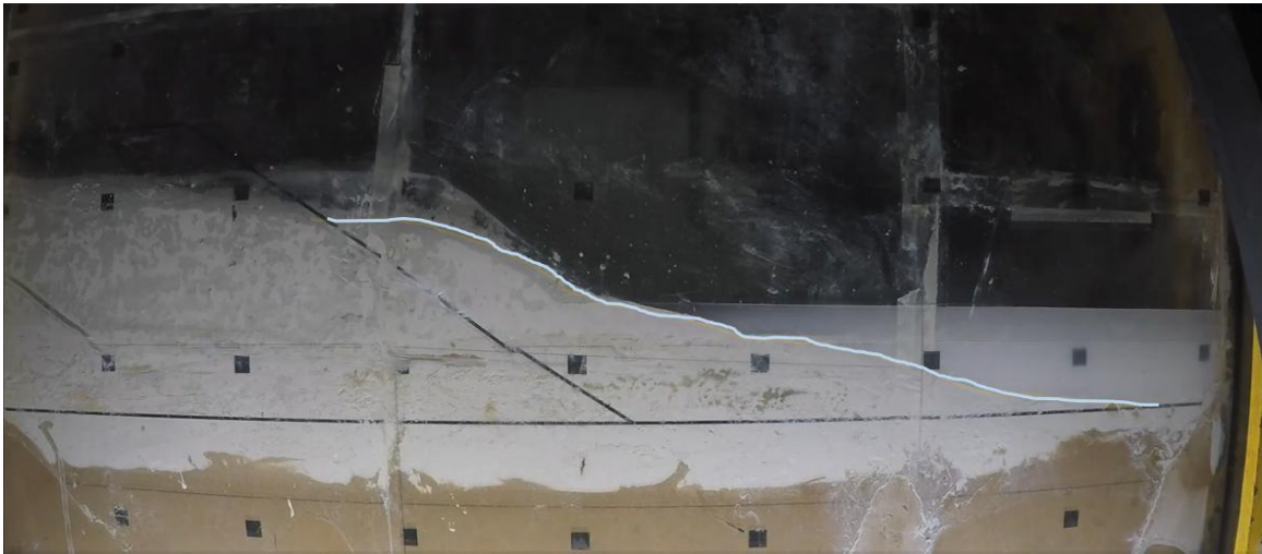
Figure 31. Time-lapse slope deformation through contour overlays from t_7 (30g) until before reaching the t_8 (30g). Start of the rain simulation.
