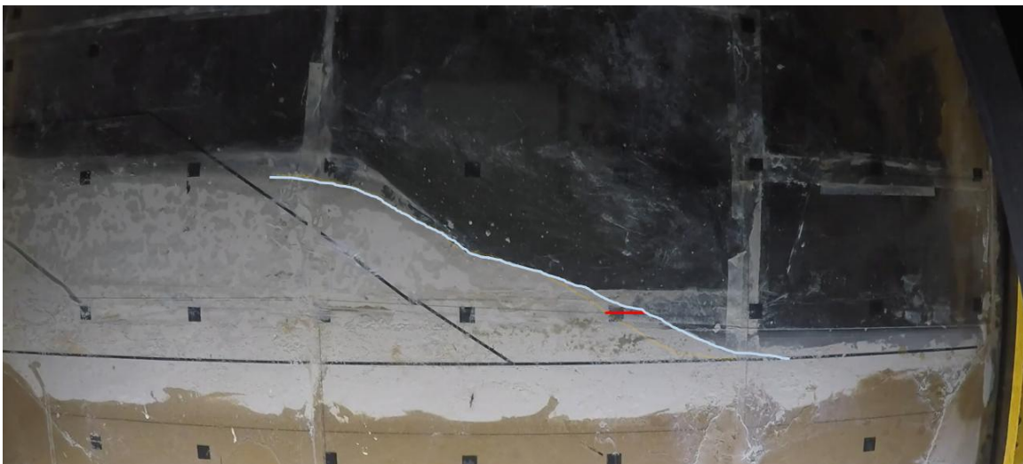
Figure 29. Time-lapse slope deformation through contour overlays from t_5 (20g) until before reaching the t_6 (25g).
