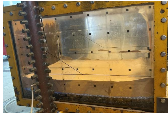
Figure 42. Experimental setup after deposition of the sand layer and initial water saturation.
