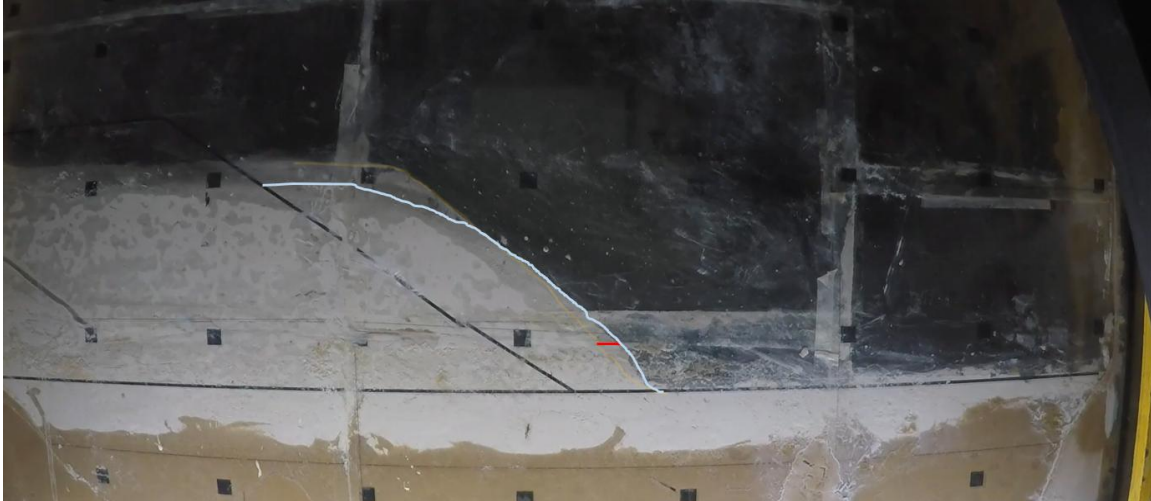
Figure 27. Time-lapse slope deformation through contour overlays from t_3 (10g) until before reaching the t_4 (15g).
