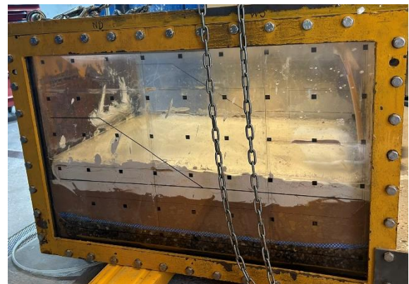
Figure 43. Experimental setup after slurry deposition of the first clay layer (70 mm thickness) and addition of water.
