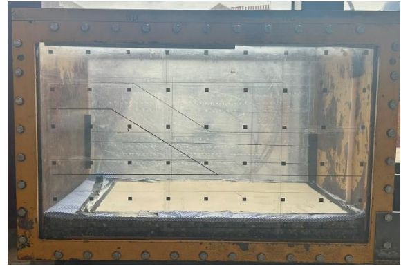
Figure 41. Experimental setup showing the drainage layer construction with gravel, filter material, and pipe installation in the centrifuge container.
