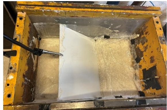
Figure 44. Experimental setup after deposition of the second clay layer (52 mm thickness), followed by placement of the upper clay slope (230 mm thickness) using plastic wall support.
