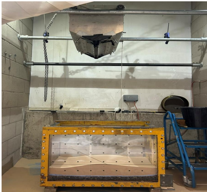
Figure 10. Sand deposited with slot pluviator at the Laboratory of Geotechnical University of Dundee.
