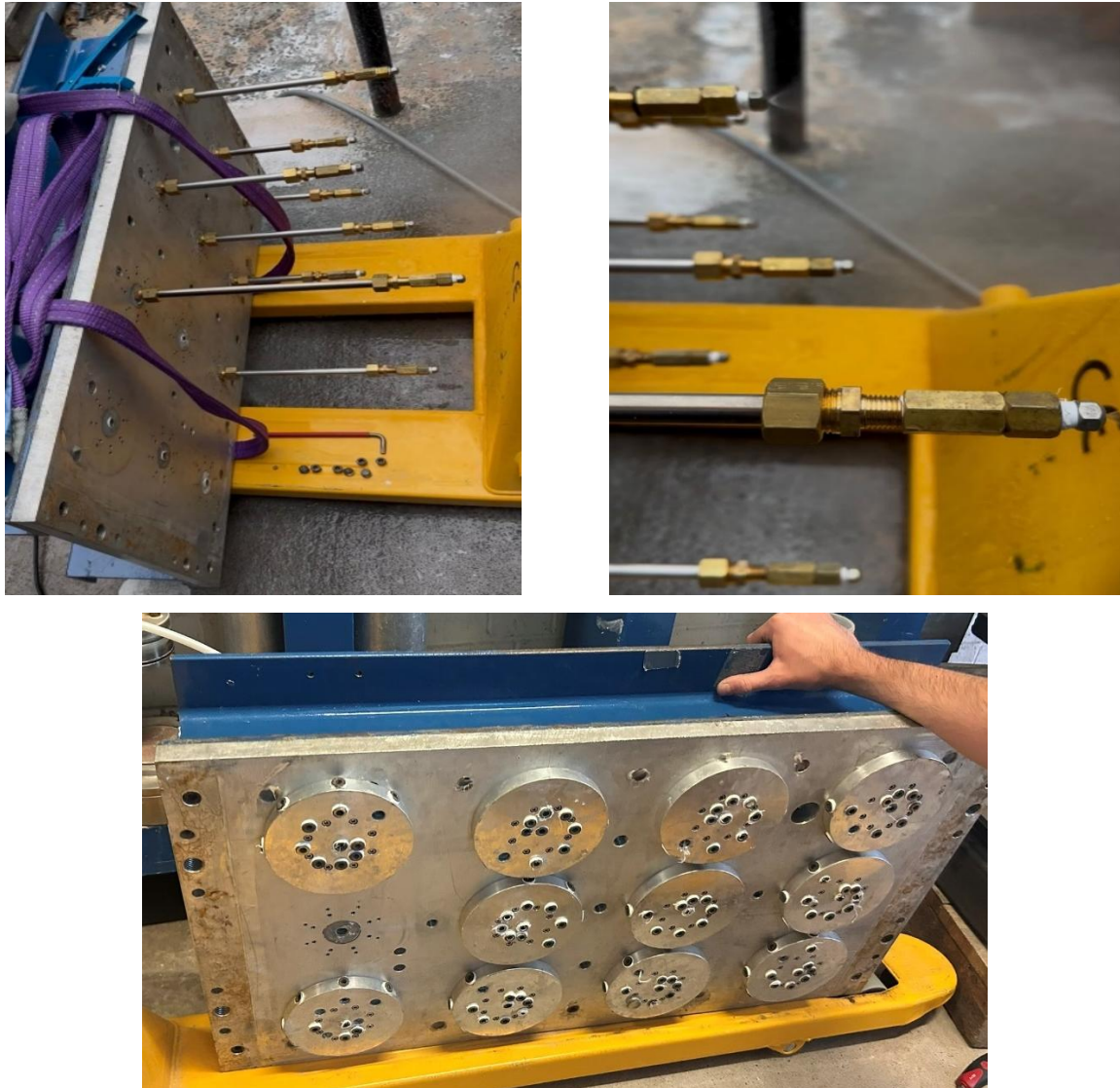
Figure 13. Rainfall equipment: aluminum lid with service ports and manifold (leak-check under pressure); distribution rail and quick-connects; eight downward-facing nozzles; assembled strongbox with rainfall rail and instrumentation mounts.
