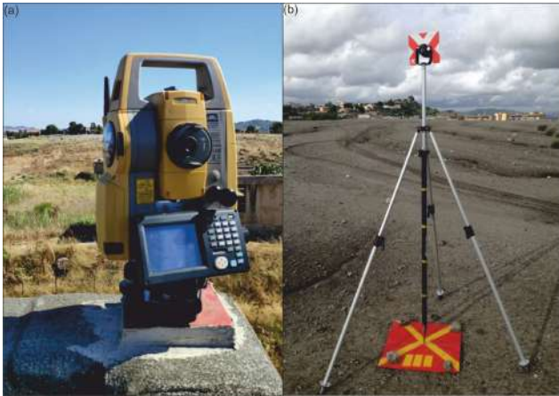
Figure 5. (a) TST DS 103 placed on the fixed metal base in coincidence with point CTN0. (b) Surveying ranging rod on the mud volcano during the survey phase.
