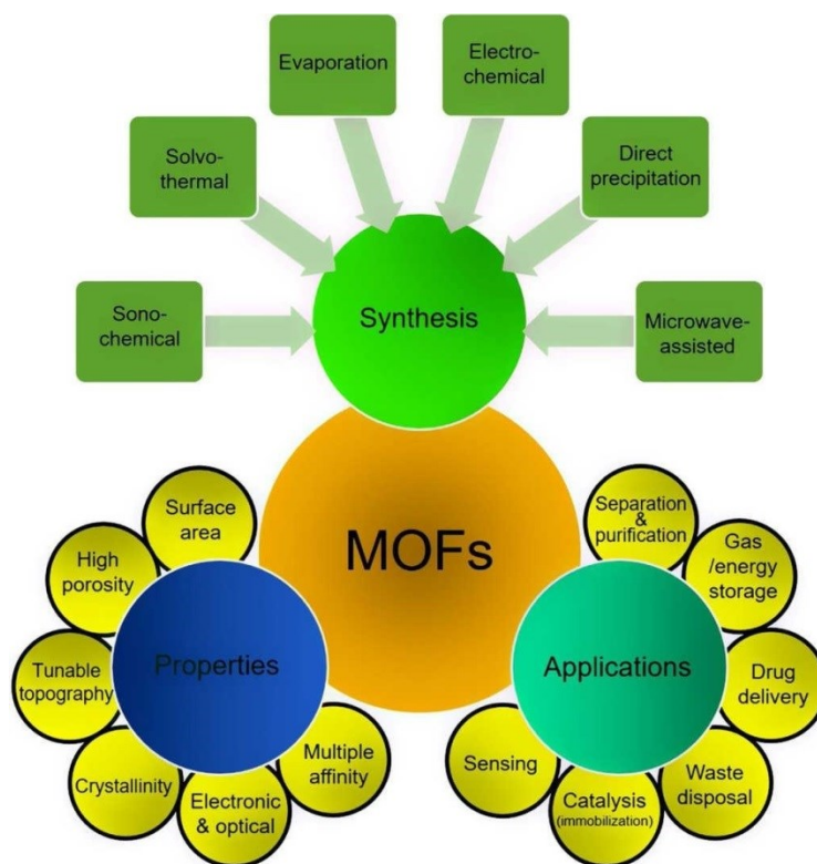
Scheme 3: Correlation between main synthetic route of MOF powders, their structural properties and possible applications. 91
