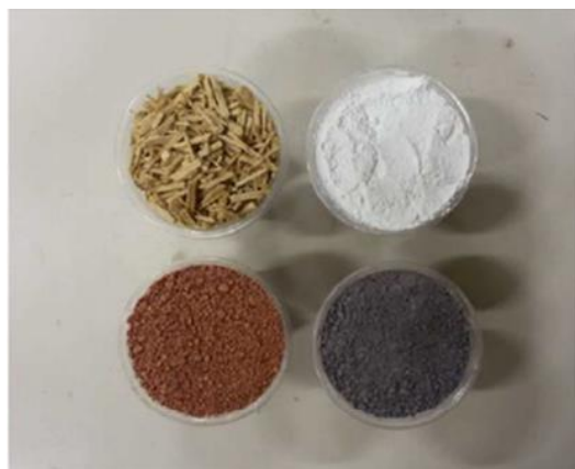
Figure 1. Main components of the cement–reed mixture. From the top, rotating clockwise: Arundo Donax, white cement, Azolo sand, Recycled clay aggregate.
