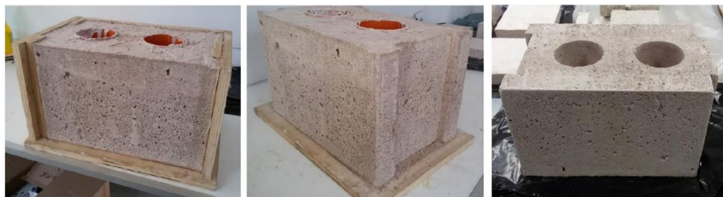
Figure 4. Prototyping of the cement–reed block.
