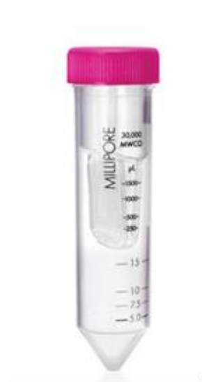
Fig. 22: Ultrafiltration and concentration system
