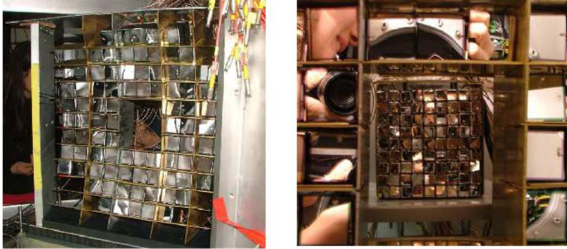
Figure 2.1.2: Left: the 88 modules of the Hodo-Big. Right: the Hodo-Small detectors arranged in a cube of 81 telescopes.
