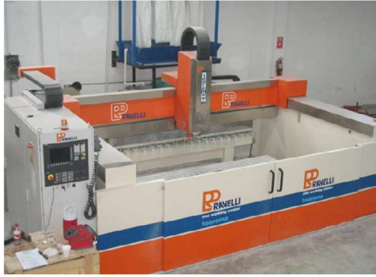
Figure 6 – Teorema SB Numerically controlled machine of the Amato Marmi company (Daniele Calderoni, 2019)
