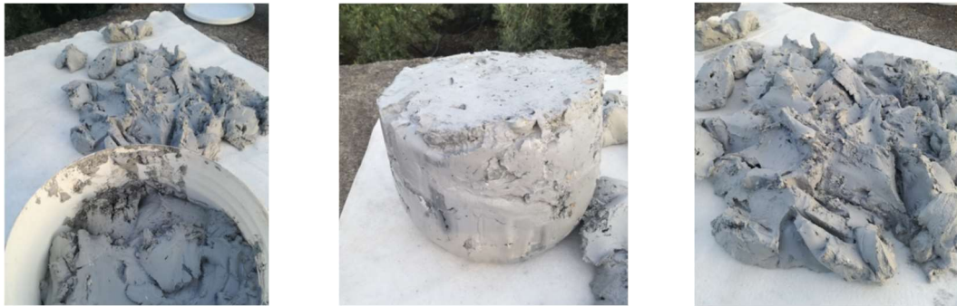
Figure 7 – Marble cutting waste natural drying process (Daniele Calderoni, 2019)
