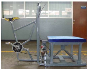
Figure 25 – Portable Shake table activated by the bicycle and technical data [34]
