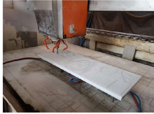
Figure 6 – Teorema SB Numerically controlled machine of the Amato Marmi company (Daniele Calderoni, 2019)
