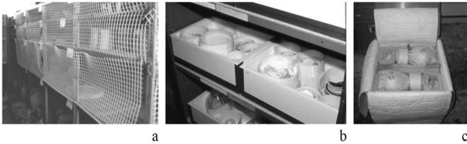
Figure 24 – Example of protection in storage areas: (a) application of mesh on the free front of the shelves; (b) wrapping objects in sheets of Ethafoam; (c) example of correct storage ). [Images from Ertürk, 2012 and Podany, 2009].
