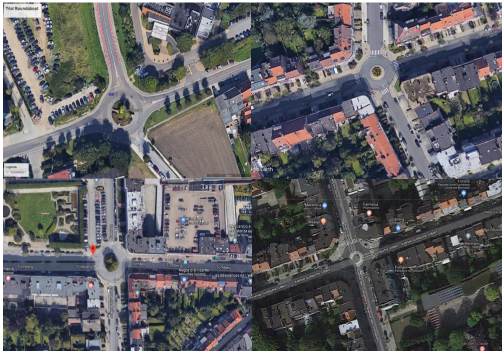
Figure 6.1– Observation sites: a) Roundabout 1 (Zaventem – D=32 meters); b) Roundabout 2 (Woluwe-Saint-Lambert – D=22 meters); c) Roundabout 3 (Tomberg – D=30 meters); d) Roundabout 4 (Ixelles – D=20 meters).
