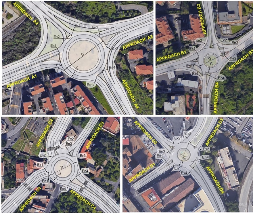
Figure 3.1 - Geometric plan views of the four roundabouts studied.
