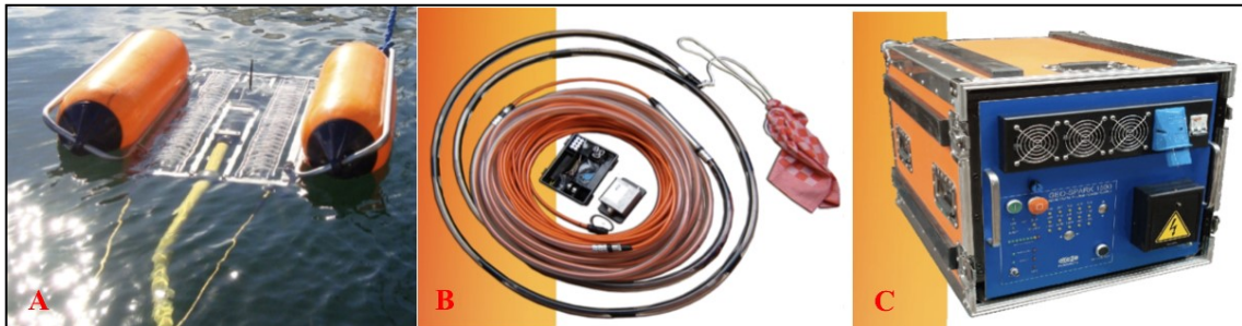
Fig. 1.9 – Main components of Marine Multi-Tip Sparker System, Geo-Source 200 Light Weight model . A. Geo-Spark 1000 Pulsed Power Supply ; B. Mini-Streamer (16 hydrophones) ; C. Solid State Pulsed Power Supplies .
