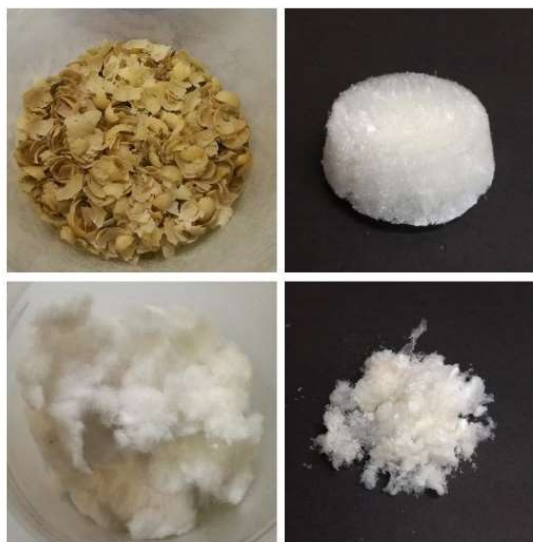
Figure 2.2 Photographs of soy hulls (top row) and cotton powder (bottom row) and their ensuing freeze-dried cellulose nanocrystals (right side).
