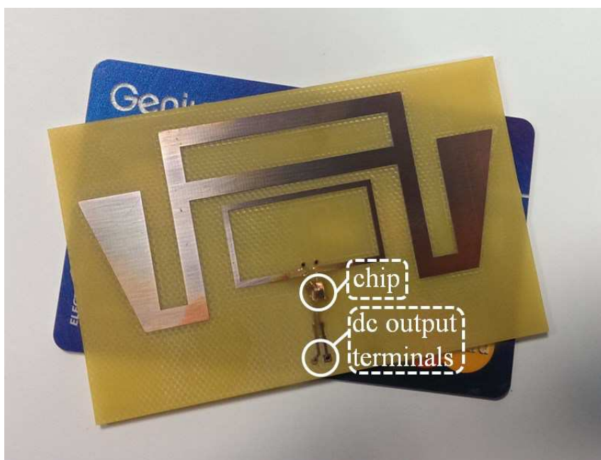
Fig. 6.3. Photograph of the fabricated ICL antenna.
