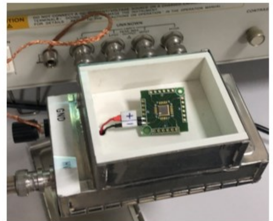
Figure 60. Two boxes used for I-V (left side) and CV (right side) measurements respectively.
