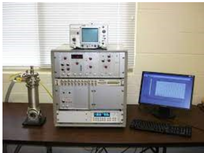
Figure 34. Typical instrument for deep level transient spectroscopy measurements.
