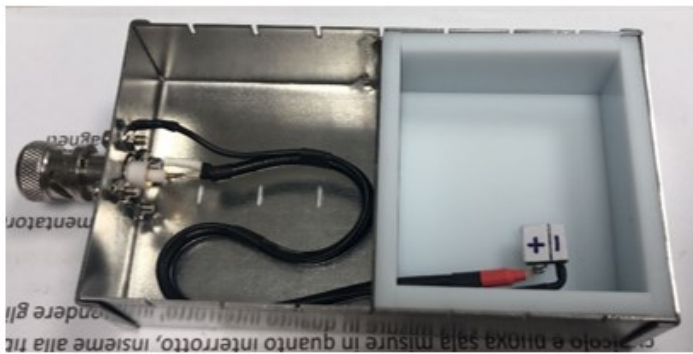
Figure 60. Two boxes used for I-V (left side) and CV (right side) measurements respectively.
