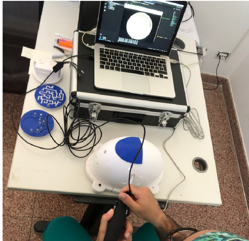
Figure 3. Arthrozero training session (ZERO group) performed on the FAST-like training module used in the study, illustrating the simulator setup and participant interaction during the task execution.
