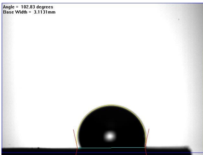
FIGURE 3.17 CONTACT ANGLE OF WATER DROP ON Pd NWS
