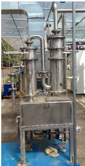
Fig.11 – Cleaning Gas Section
