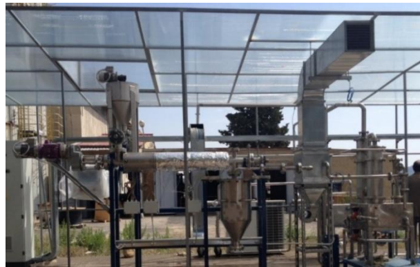
Fig.6 – Macro of Pyrolysis Pilot-Plant [87]
