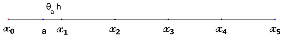
Figure 1.3: Discretization of the domain [\mathbf{a}, \mathbf{b}] with n = 5 : the black dots are the internal points , the red dot is the only ghost point . We impose the Dirichlet boundary conditions in the blue dots \mathbf{a} and \mathbf{b}=x_5=1
