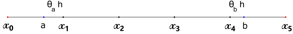
Figure 1.6: Discretization of the domain [\mathbf{a}, \mathbf{b}] with n = 5 : the black dots are the internal points , the red dots are the two ghost points . We impose the Dirichlet boundary conditions in the blue dots \mathbf{a} and \mathbf{b}
