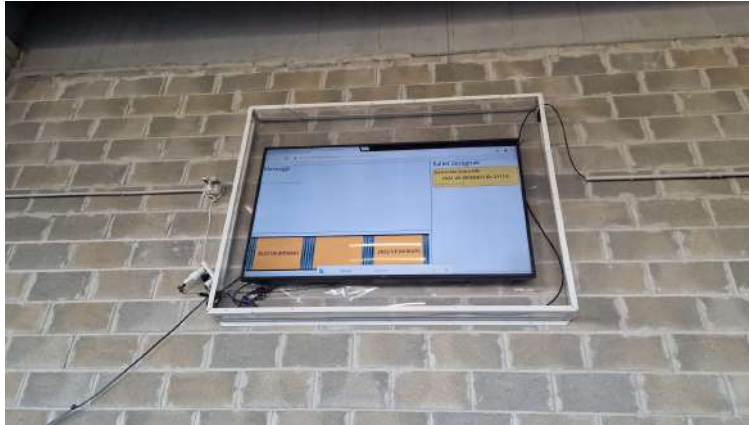
FIGURE 3.13: Monitors installed in the loading area where delivery staff can see which pallets are traveling on the roller conveyor.
