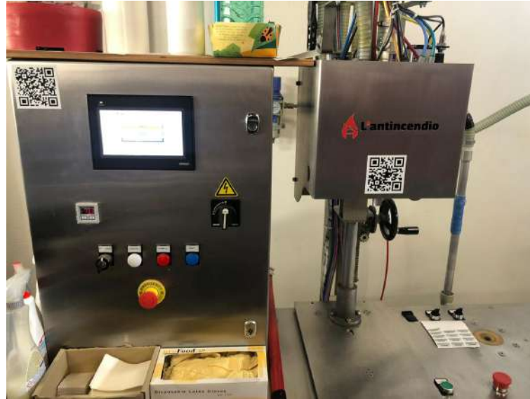
FIGURE 3.6: A picture of the new machinery for the maintenances of the powder extinguishers.
