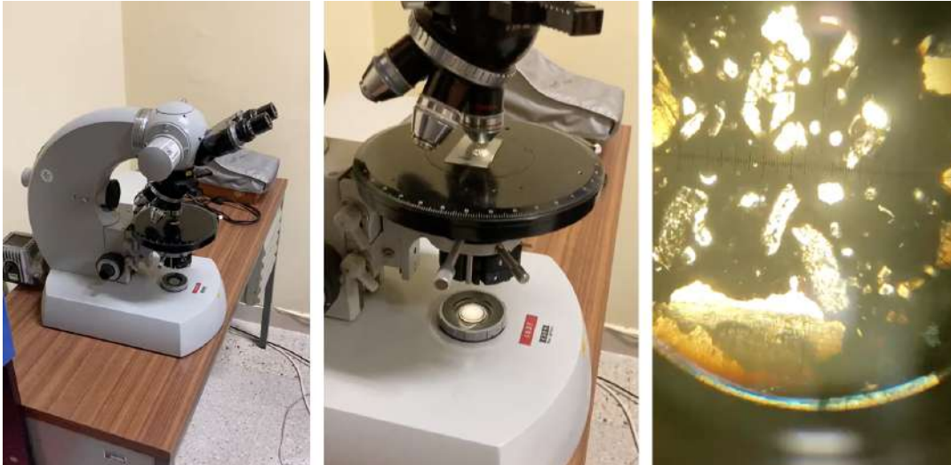
FIGURE 4.5: Microscope and observation of a basalt thin section at low magnification through the eyepieces of the microscope.
