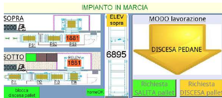
FIGURE 3.10: State of the pallet moving system from the HMI. PS1, PS2 and PS3 are the upper floor stations. The lift position is represented with a value between 0 and 6895. PI4, PI3, PI2 PI1 are the lower floor stations.
