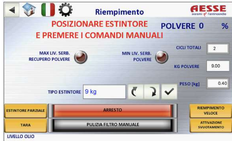
FIGURE 3.7: A screen took for MAS 4.0 HMI where is possible to see the recipes, configuration and alerts.
