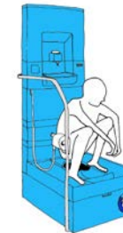
3. Do „your business“ in a way that feces and urine are separated
