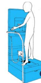
5. Push the flush button. The lid to the feces opening closes automatically
