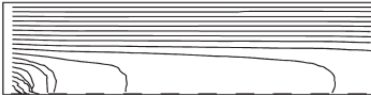
Fig. 1.3 Particle trajectories in a medium liquid in the device operating in p-DEP condition only at the bottom of the channel. (Figure taken from: F. Aldaeus, Y. Lin, J. Roeraade, and G. Amberg, Electrophoresis 26 , 2005).
