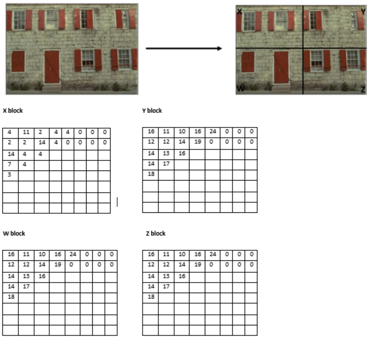
Figure 4.8: An image with a cut and paste operation performed on the second quadrant of the image between first and second compression. Only the quantization table of the first block changes.
