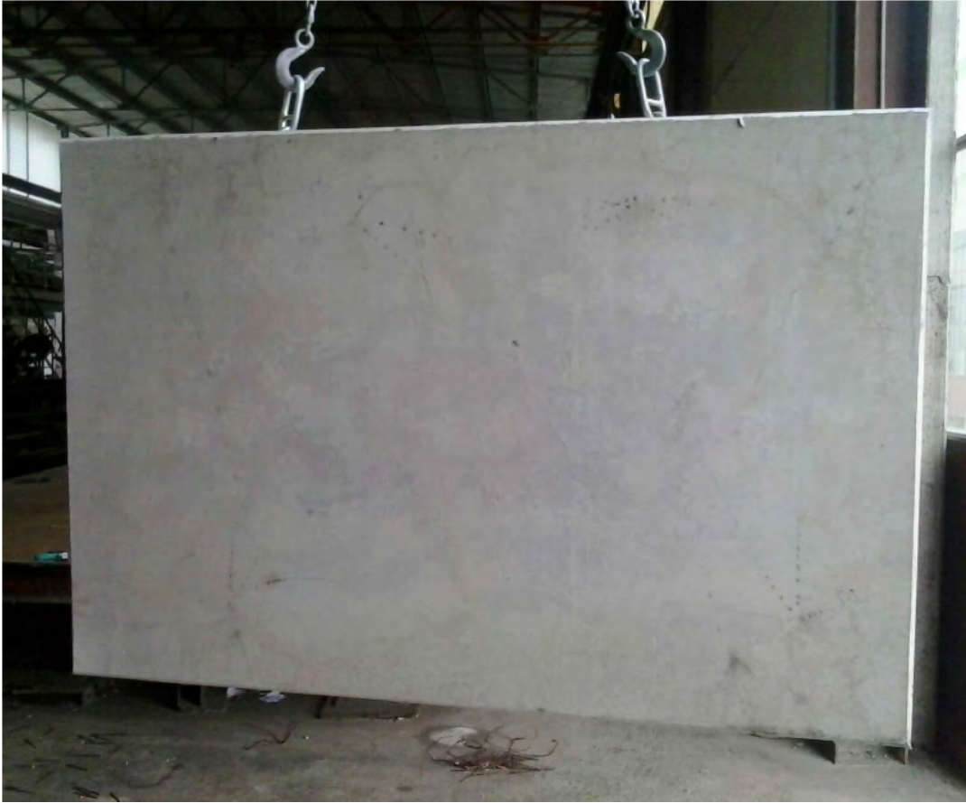
Fig. 4 - Precasted panel made with foam glass from recycling (credits: SAM Engineering spa).
