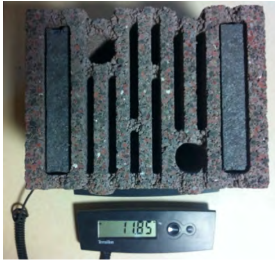
Fig. 3 - Block made with foam glass from recycling (credits: UNIBLOC srl).
