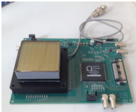
Fig. 3. – A front-end (FE) board equipped with a Hamamatsu H8500 64 channel PSPM and a MAROC3 chip.
