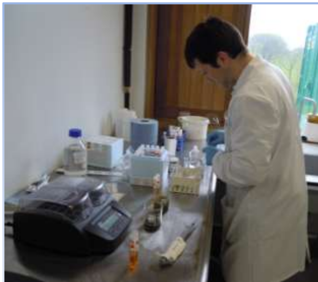
Figure 2.3.2. Preparation sample for COD and \text{NH}_4^+ determination
