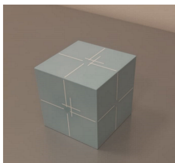
Figure 4. WL3 Varian Mobius Phantom for Winston-Lutz test.
