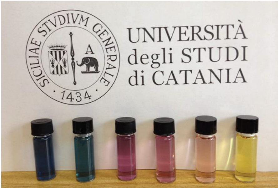
Fig.10: Different anisotropic AgNPs. The macroscopic coloration is an indication of a change in the plasmon resonance peak.
