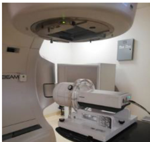
FIGURE 2 myQA SRS high-resolution detector (IBA dosimetry).
