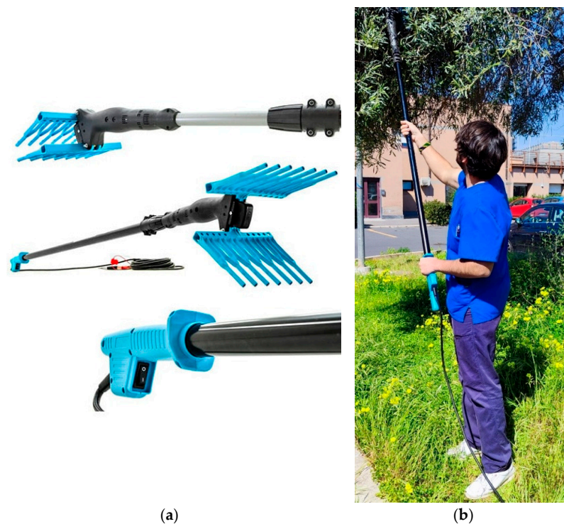
Figure 1. Olive harvester (model: CILLI B-140) (a); operator using the electric olive harvester (b).
