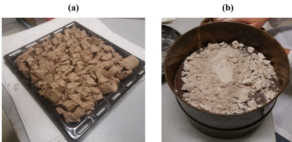
Figure 10 - GSW as received before the drying process (a); and after drying while sieving (b).
