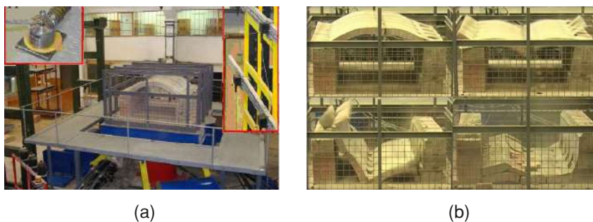
Fig. 2.7: Seismic tests on GFRP reinforced masonry vault (adaped from Taranu et al. [2010]): (a) testing setup conditions, (b) collapse phases
