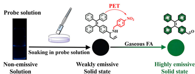
Fig. 1 Preparation of TPE-FA in the solid state and variation in emissions in response to gaseous FA. Reproduced from ref. 36 with permission from the American Chemical Society, copyright 2018.
