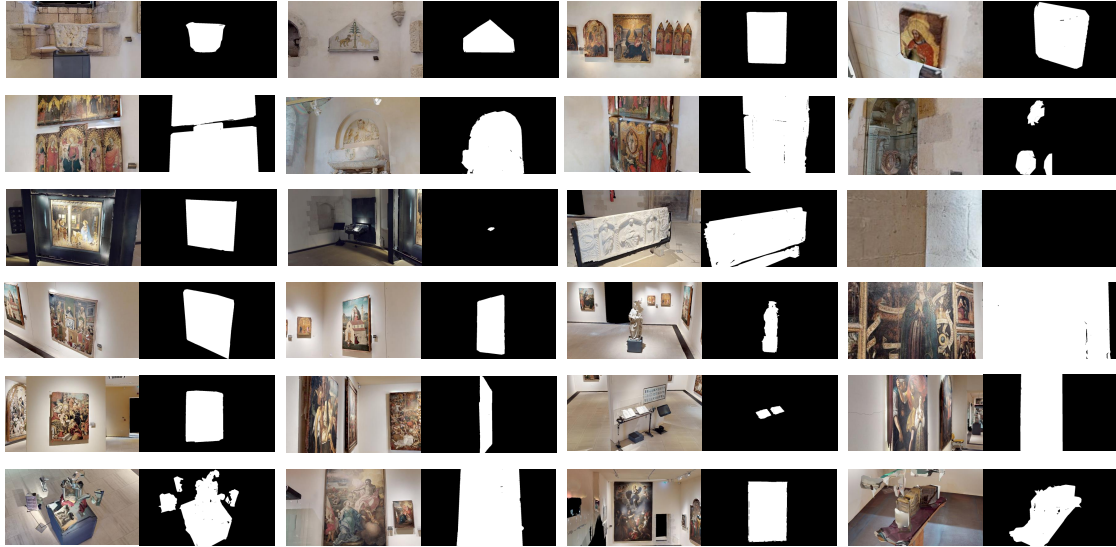
Figure 3.27: Samples of synthetic images of the 24 artworks with the related segmentation masks automatically generated using the developed tool.
