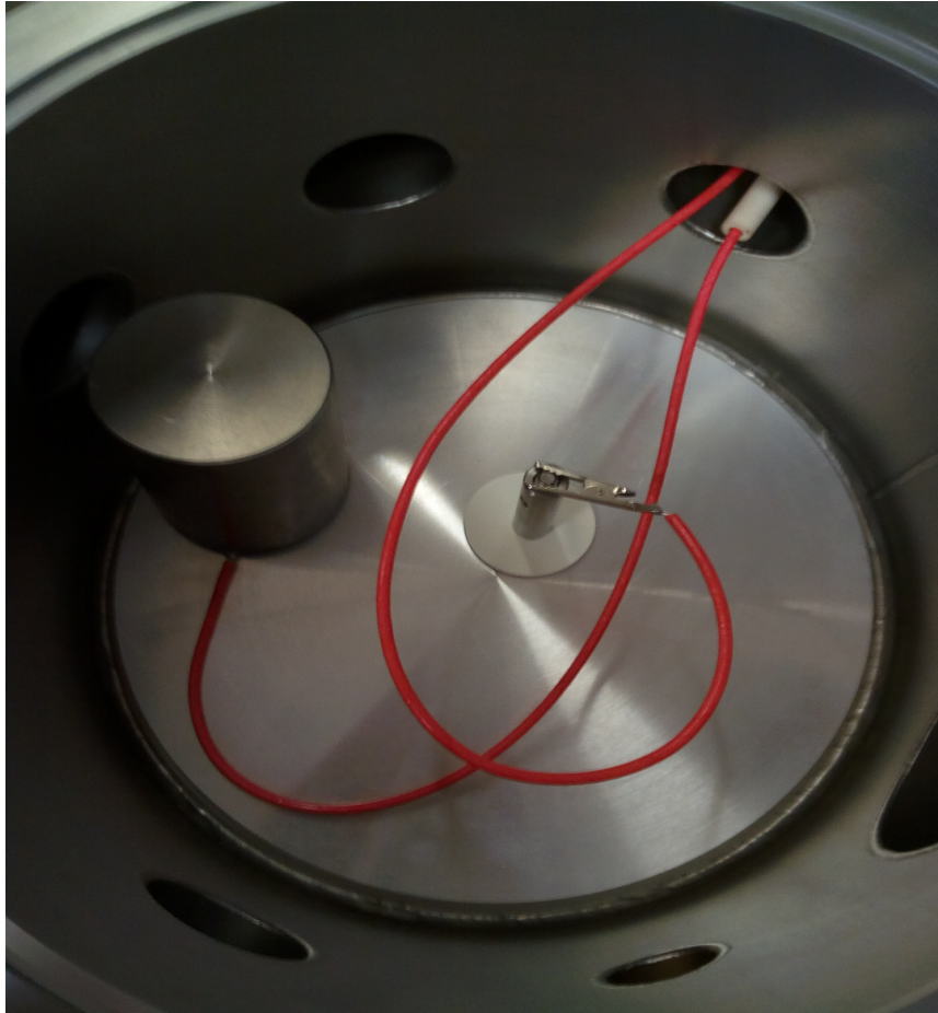
Figure 5.54: PBN sampe placed in a small vacuum chamber, a standar post from ThorLab is used as electrode connected with the power supply
