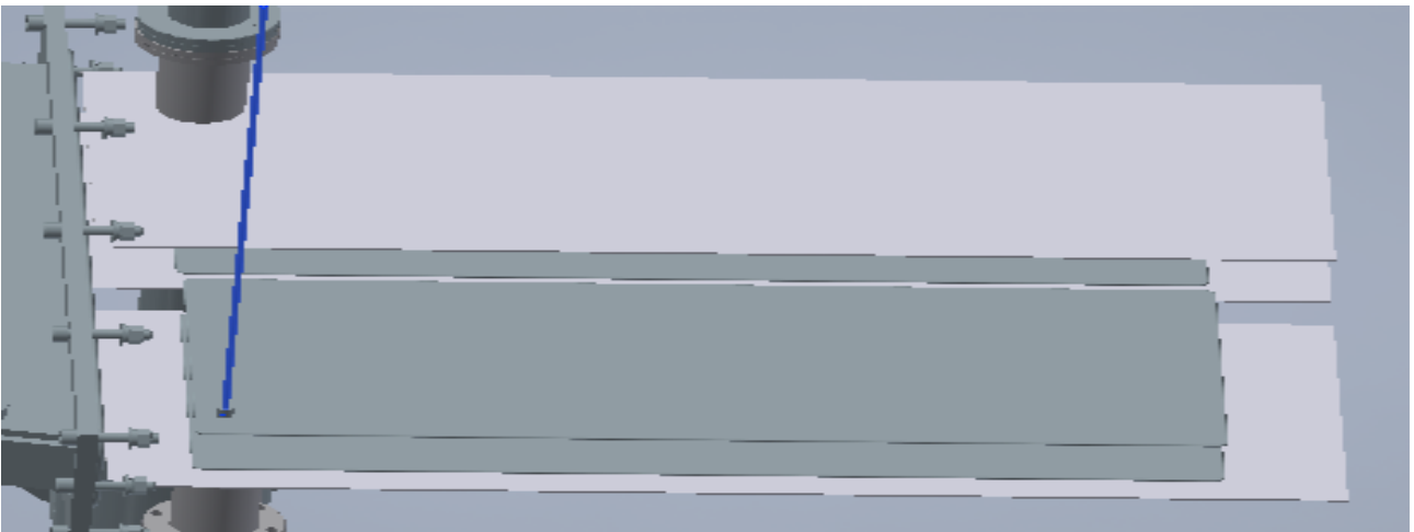
Figure 5.17: Details of the electrodes (dark gray) and insulator (light gray), in blue is shown a portion of the HV wire
