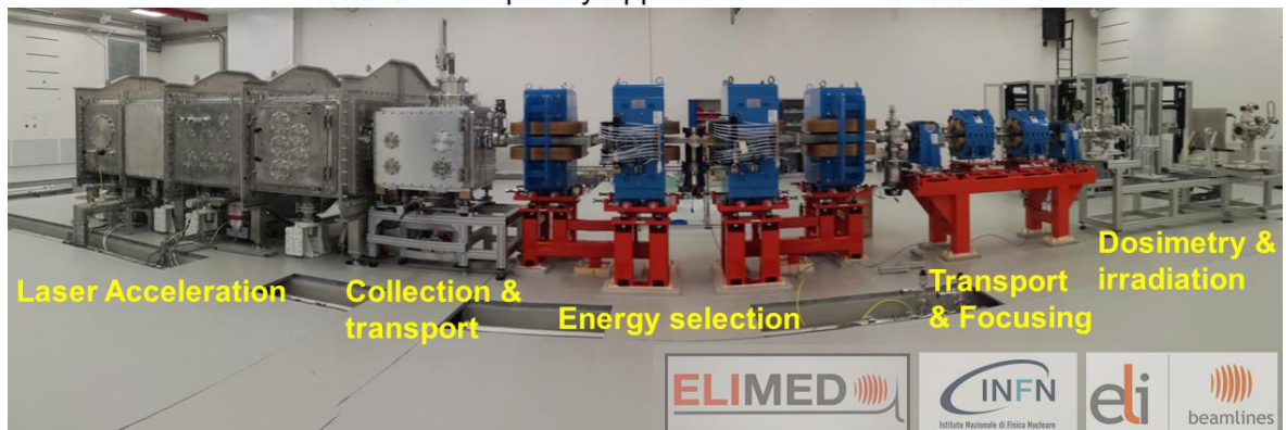
Figure 1.12: The main sections of the ELIMAIA beamline (Ion Accelerator and ELI MEDical applications (ELIMED)) consist of different subsystems: (i) acceleration, collection and diagnostics; (ii) collection, selection and transport; (iii) dosimetry and sample irradiation.
