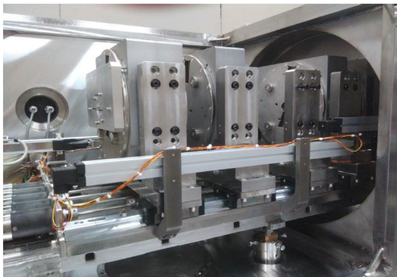
Figure 2.32: PMQs with mechanics installed at INFN-LNS
