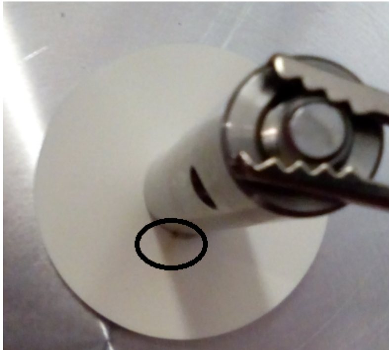
Figure 5.56: PBN sample after test, the burn due to the discharge between the glue and the electrode circled in black
