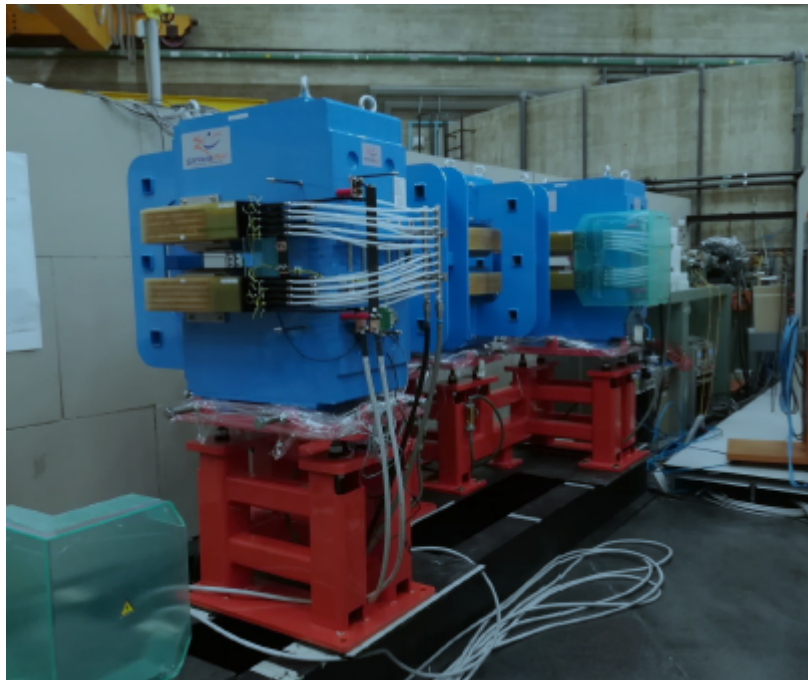
Figure 3.49: Energy selector installed at the 40° beamline
