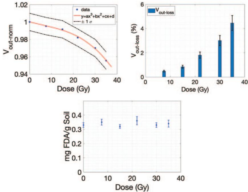
Fig. 3. – Top left:  $V_{out-norm}$  as a function of the absorbed dose (blue dots), with the relative  $\pm 1\sigma$  band (black dashed line), and the results of the third-degree polynomial regression (red line). Top right: percentage of  $V_{out-loss}$  as a function of the absorbed dose. Bottom: FDA activities expressed as mg FDA per g of soil, as a function of the absorbed dose.
