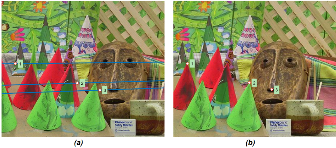
Figure 8: Considering any point in the right image (b) I_R (1, 2 and 3), the method in [22] searches the corresponding points in the left image I_L by computing their epipolar lines (a).
