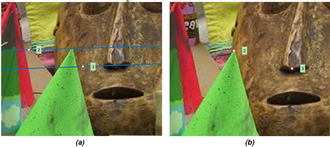
Figure 9: Details of the images shown in Figure 8. The tip of the cone (i.e., point number 2 in the image (b) depicting the right view I_R ) corresponds to a point that lies on the corresponding epipolar line (i.e., line number 2 in (a)) on the left view I_L .
