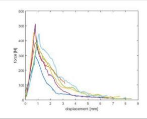
**Figure 10.** Typical set load-displacement curve for reinforced samples  $(F-\delta)$ .
