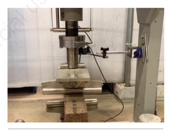
Figure 4. A sample ready for the flexural test.
