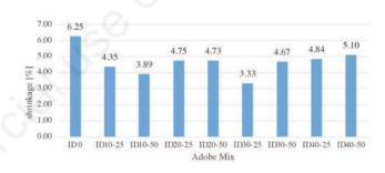
Figure 9. Shrinkage rate for prismatic samples.
