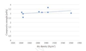
**Figure 8.** Correlation between dry density and compressive strength.
