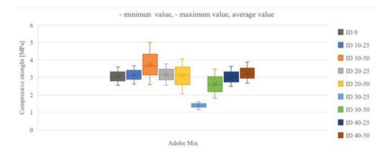
Figure 7. Average values of compressive strength of the adobe mix, including minimum and maximum values for each mix.
