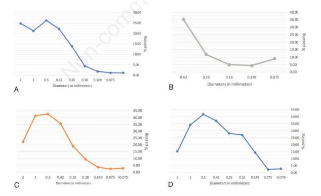
Figure 1. Particle size distribution of Floridia soil (FS) (A), clay (B), the size distribution of FSM (C), the particle size of the final mix (including sand) (D).
