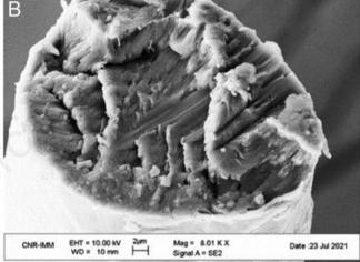
Figure 2. Scanning electron microscope analysis of sheep wool fibre surface (A) and transversal section (B).
