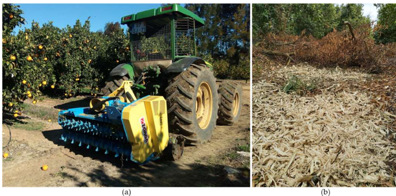
Figure 18. Shredding of pruning residues. (a) Shredder working in a citrus orchard. (b) Pruned branches before and after shredding.
