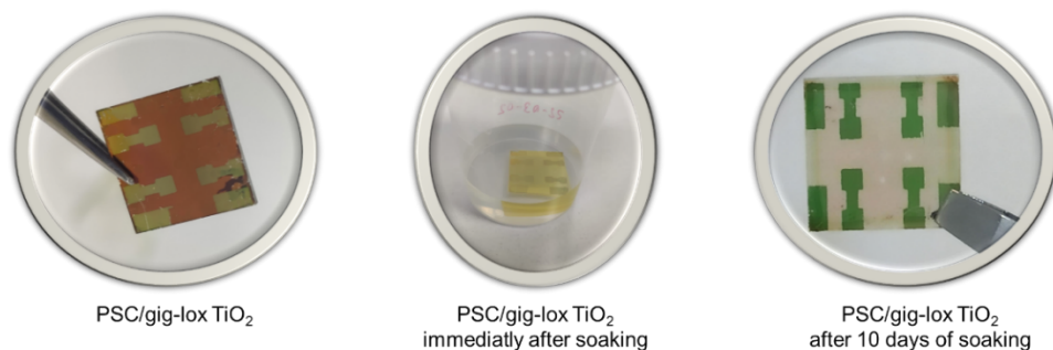
Figure A4.3 Photos of a representative PSC/gig-lox \text{TiO}_2 sample before, immediately after soaking and after 10 days of soaking in water ( \text{pH} \sim 5.8 ).
