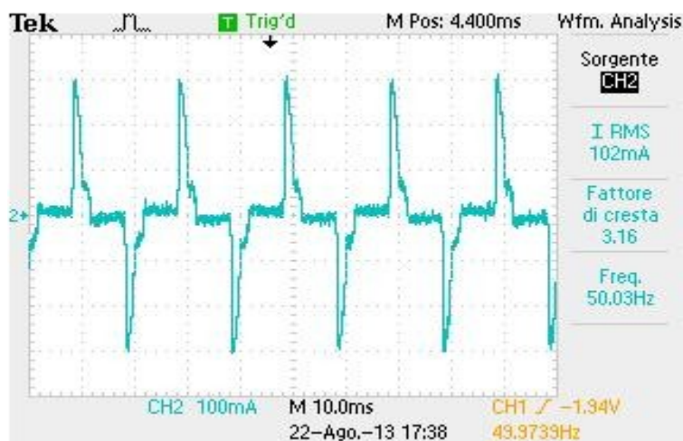
Fig. 5.2 Waveform of the current drawn by the lamp CFL
